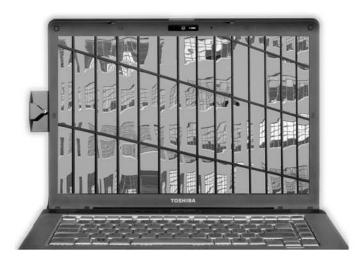
Viewing Angle Gauge installed on a laptop computer.
