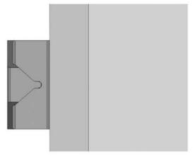
This is what the Viewing Angle Gauge looks like when you are viewing it at the correct angle.
